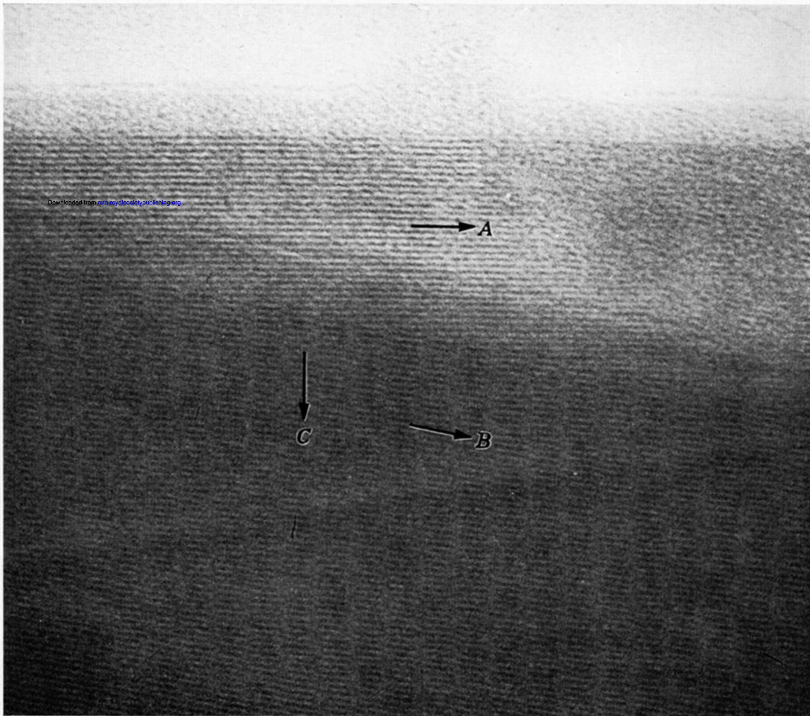
FIGURE 19. Overlapping crystals of platinum phthalocyanine showing crystal lattice fringes resolved and a moiré pattern formed in the region of overlap. (Magn. \times 950\,000 .) (Courtesy Menter 1958.)
