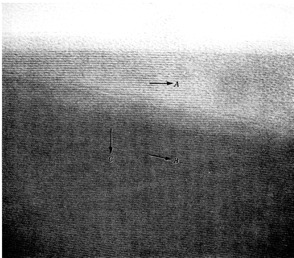
FIGURE 19. Overlapping crystals of platinum phthalocyanine showing crystal lattice fringes resolved and a moiré pattern formed in the region of overlap. (Magn. \times 950\,000 .) (Courtesy Menter 1958.)
